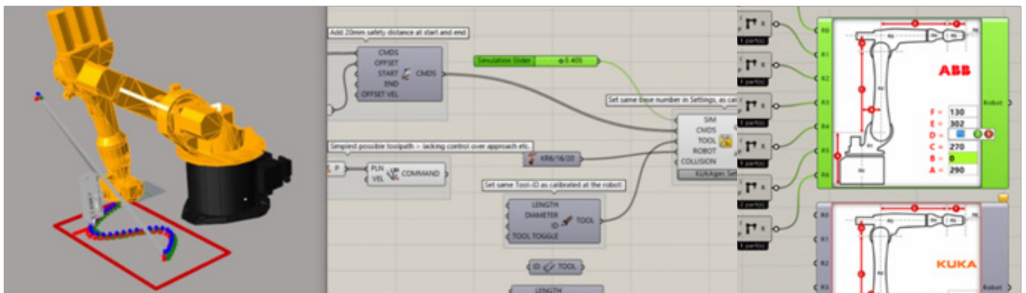
Figure 2: Robotic control using Grasshopper Plug-ins
